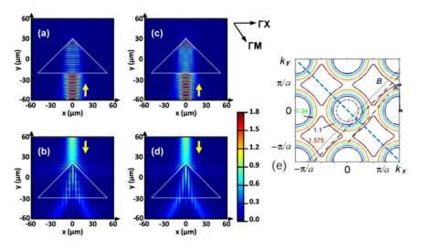
Fig. 6. Electric field distributions at 64 THz (ka = 1.34): for PhC prism at (a) forward-case (here - normal,  $\Gamma X$  interface) illumination and (b) backward-case (here - wedge) illumination, and for solid dielectric prism with n = 1.68 at (c) forward-case (here - normal, longer-side) illumination and (d) backward-case (here - wedge) illumination; yellow arrows show directions of beam incidence; (e) EFCs in ( $k_x, k_y$ )-plane and construction lines: solid lines -
