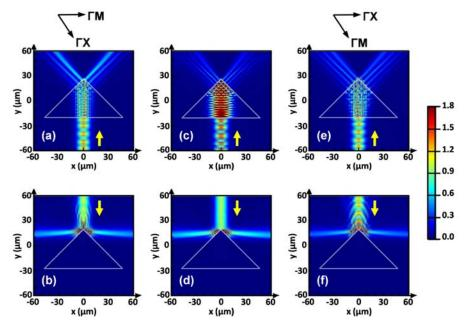
Fig. 3. Electric field distribution at 179 THz (ka = 3.75): for PhC prism at (a) forward-case (here -  $\Gamma M$  interface) illumination and (b) backward-case (wedge) illumination; for non-magnetic ULIM prism with n = 0.22 at (c) forward-case (here – longer-side) illumination and (d) backward-case (wedge) illumination; for PhC prism at (e) forward-case ( $\Gamma X$  - interface) illumination and backward-case (wedge) illumination; yellow arrows show directions of beam incidence.
