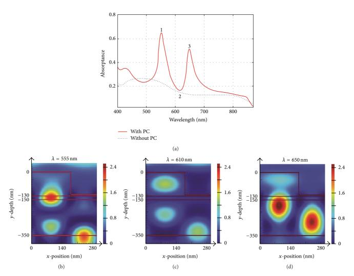
FIGURE 4: Calculated absorptance spectrum and optical field intensity distribution for a solar cell structure with the following parameters: 20 nm-thick InGaN layer, 130 nm-thick GaN cap layer, 300 nm lattice length, 50% fill factor, and 120 nm etch depth. (a) Calculated absorptance. (b) Field distribution at 555 nm wavelength. (c) Field distribution at 610 nm wavelength. (d) Field distribution at 650 nm wavelength.
