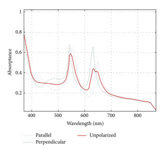
FIGURE 2: Calculated absorptance spectra for an optimized (FF = % 50, h = 130 nm, and a = 300 nm) solar cell structure with a 130 nm-thick GaN cap layer and a 20 nm-thick InGaN layer in the case of parallel (blue dotted), perpendicular (green dashed) polarizations with respect to the photonic crystal pattern, and unpolarized light incidence (solid red).
