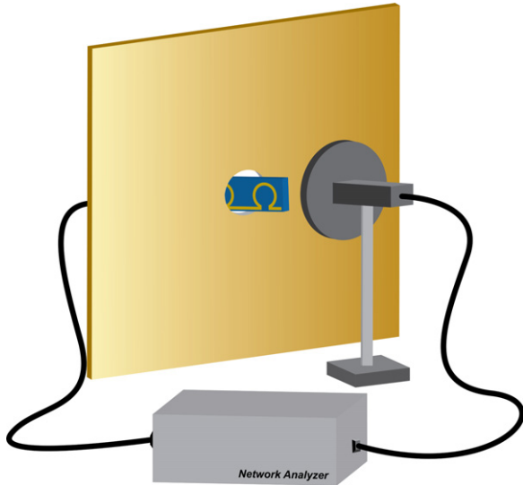
Fig. 2. Schematic demonstration of the transmission enhancement experiments using open-ended waveguide antennas and the HP8510C network analyzer.
