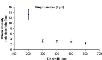
Figure 6 SERS intensity ratio depending on slit-width changes.
