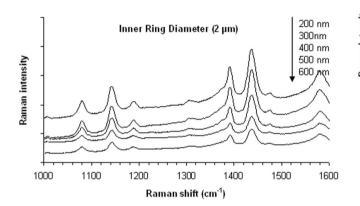
Figure 5 SERS spectra obtained from plasmonics lenses with different slit widths.
