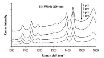
**Figure 7** SERS spectra obtained from plasmonic lenses having the same slit width with different ring diameters.
