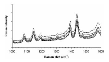
**Figure 3** Ten SERS spectra obtained from the equivalent plasmonic lenses on the same array.
