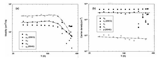
**Fig. 3** (a) Mobility and (b) carrier density versus temperature. The closed circles represent the measured mobility and carrier density taken at 0.5 Tesla. The triangles represent the extracted 2DEG mobility and carrier density. The open circles represent the extracted 2DHG mobility and carrier density. The stars and squares represent the bulk carriers. The lines are guide for the eyes.
