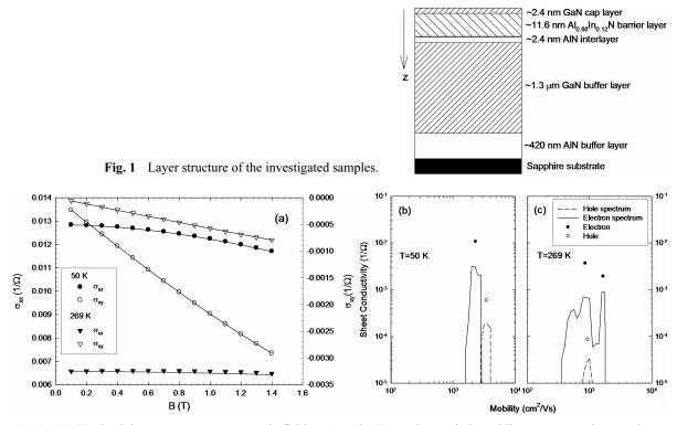
**Fig. 2** (a) Conductivity tensors versus magnetic field at 50 and 269 K. The symbols and lines represent the experiment and QMSA fits, respectively. Mobility spectra obtained with using QMSA at (b) 50 K and (c) 269 K. Calculated carriers are shown with symbols.
