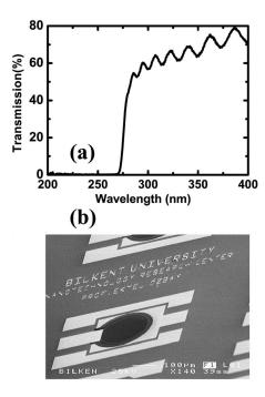
FIG. 1. (a) Spectral transmission of the wafer that was used in the fabrication of the detectors and (b) scanning electron microscopy image of 200  $\mu$ m diameter fabricated devices.
