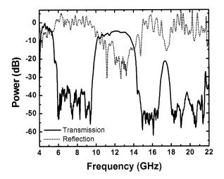
Fig. 4. Measured transmission and reflection spectra of the DNG composite metamaterials. Relatively high power, — 4.5 dB, is measured between frequencies 9.5 and 14.5 GHz in which both effective permittivity and permeability have negative values. The reflection spectrum also has average — 20 dB rejection throughout this region.
