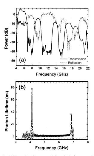
Fig. 2. (a) Measured broad-range transmission and reflection spectra of the SRR medium along  $\boldsymbol{x}$  direction in free space. The transmission spectrum exhibits series stopbands and passbands. The negative permeability regions do not allow the propagation of electromagnetic waves through the SRR structure. (b) Measured delay time, photon lifetime, as a function of frequency. The delay time increases rapidly as we approach the band edges.
