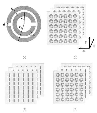
Fig. 1. (a) A single copper SRR with parameters  $r_1=2.5$  mm,  $r_2=3.6$  mm, d=w=0.2 mm, and t=0.9 mm. Schematic drawing of (b) the negative  $\mu$  medium, (c) the negative  $\varepsilon$  medium, and (d) the composite DNG metamaterial.
