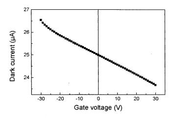
FIG. 8. Theoretical dependence of the dark current, flowing through the PbS layer, on the gate voltage applied on the Si substrate. Equation (3) was used, with  $X_{PbS}$  given by Eq. (5). Values used for the simulation:  $V_d = +30$  V,  $R_L = 1$  M $\Omega$ , and  $V_g$  varied between -30 and +30 V.
