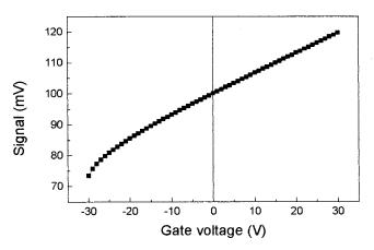
FIG. 9. Theoretical dependence of the photoconductive signal on the gate voltage, obtained using Eq. (6), for a wavelength that is uniformly absorbed in PbS. Values used for the simulation:  $V_d = +30$  V,  $R_L = 1$  M $\Omega$ , and  $V_g$  varied between -30 and +30 V.
