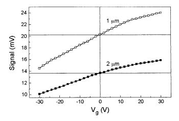
FIG. 5. Dependence of the photoconductive signal on the gate voltage  $(V_d = +30 \text{ V})$ .
