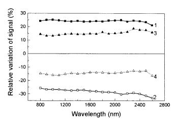
FIG. 4. Spectral distribution of the relative variation of the photoconductive signal: (1)  $V_d = +30$  V and  $V_g = +30$  V; (2)  $V_d = +30$  V and  $V_g = -30$  V; (3)  $V_d = -30$  V and  $V_g = +30$  V; and (4)  $V_d = -30$  V and  $V_g = -30$  V. Formula (2) was used for computation.
