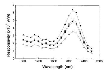
FIG. 3. Spectral distribution of responsivity in the case of PbS/SiO<sub>2</sub>/Si heterostructures, for different gate voltages: open-squares, floating gate; solid squares, ground gate; solid triangles,  $V_g = +30$  V; and open triangles,  $V_g = -30$  V. Drain voltage was +30 V.
