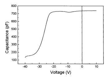
FIG. 7. C-V characteristic of the PbS/SiO<sub>2</sub>/Si structure measured at 10 kHz.
