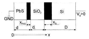
FIG. 6. Schematic of the PbS/SiO<sub>2</sub>/Si structure with voltage  $V_g$  applied on the gate electrode.  $d_1$  is the thickness of the insulating layer, *D* is the thickness of the Si substrate, and  $x_{Si}$  is the thickness of the space-charge region in Si.
