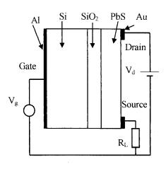
FIG. 1. Schematic of the pseudo-MOS PbS/SiO<sub>2</sub>/Si structure and of the electrical setup used for field-effect-assisted photoconductivity measurements:  $V_d$ , drain voltage;  $V_e$ , gate voltage; and  $R_L$ , load resistance.
