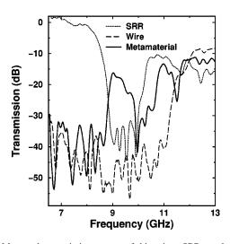
FIG. 3. Measured transmission spectra of thin wires, SRRs, and the composite structure with the second type of metamaterial configuration [Fig. 1(c)]. A transmission band is observed within the stop bands of wire and SRR structures.
