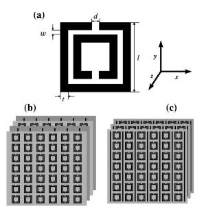
FIG. 1. (a) A single SRR with parameters  $\ell = 3 \text{ mm}$  and d = t = w= 0.33 mm. (b)-(c) Schematic drawing of two different configurations of the composite medium consisting of thin wires and SRRs.
